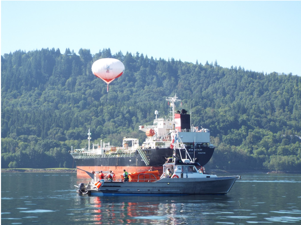
Figure 16 - Aerostat Being Operated From a Vessel
