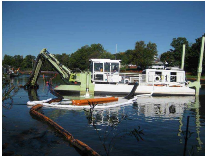
Figure 29 – Amphibex environmental dredger. Source: USEPA
