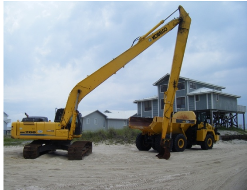
Figure 30 – Long-reach excavator for submerged or sunken oil nearshore. Source: M.W. (Mac) McCarthy
