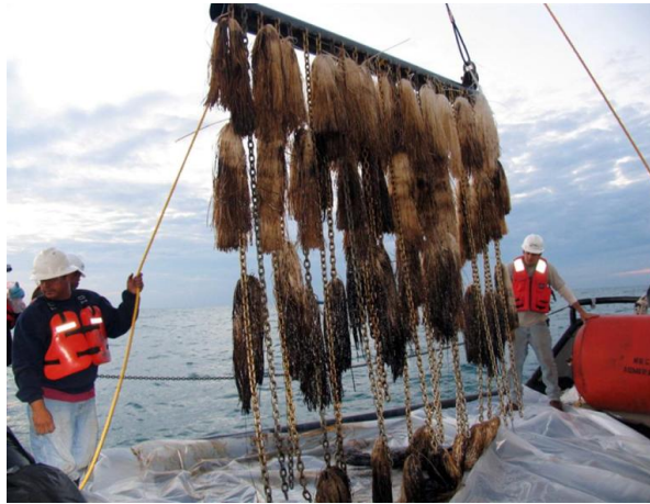
Figure 18 – Weighted sorbent sentinel array. Source: NOAA
