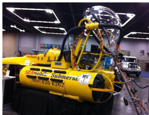
Figure 31 – Marine Pollution Control's manned submersible for the detection and recovery of submerged or sunken oil. Source: NOAA
