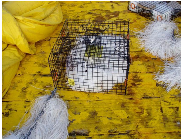
Figure 17 – Crab pot stuffed with viscous oil snare to make a passive oil sentinel. Source: NOAA
