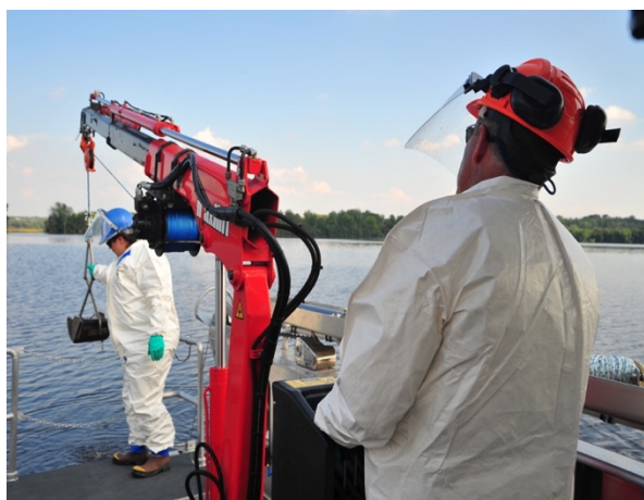
Figure 19 – Using a clamshell device to gather sediment samples. Source: USEPA
