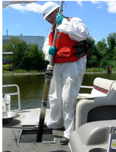
Figure 20 – Using a push core to gather soft sediment samples. Source: USEPA
