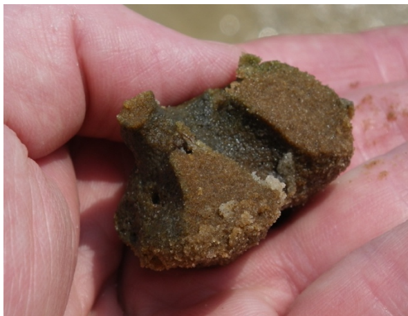
Figure 24 – Irregularly shaped tarballs often indicate offshore submerged or sunken oil mats. Source: M.W. (Mac) McCarthy
