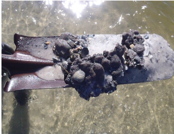
Figure 15 – Submerged or sunken oil and shell hash recovered by snorkel SCAT. Source: Polaris Applied Sciences
