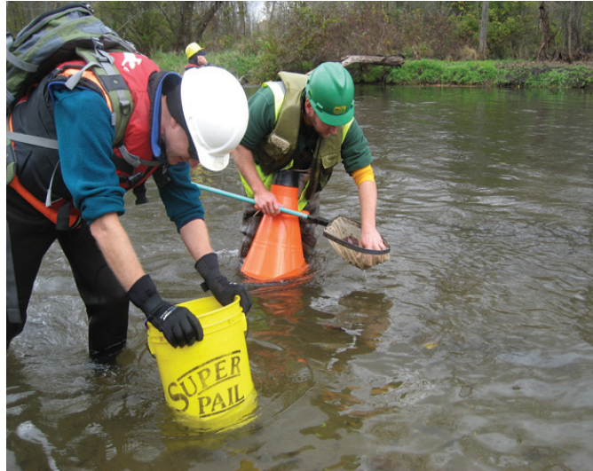
Figure 12 – Responders using view tubes to assess submerged or sunken oil. Source: NOAA
